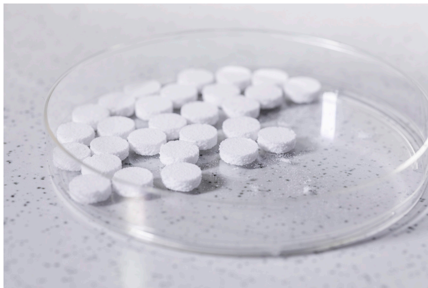
Image 2: 3D-printed lactose-starch tablets, developed by DFE Pharma. Copyright: DFE Pharma; courtesy of Netherlands Organisation for Applied Scientific Research (TNO)
