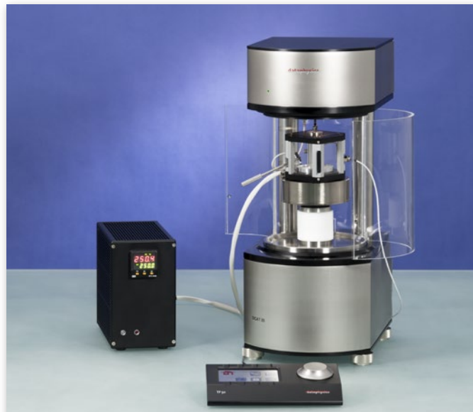
high temperature surface tension measurement with a DCAT 25
