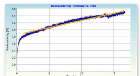
Fig. 5: mean relative backscattering intensity of the 1 st section vs. time (increase rate: 0.04 %/d)
