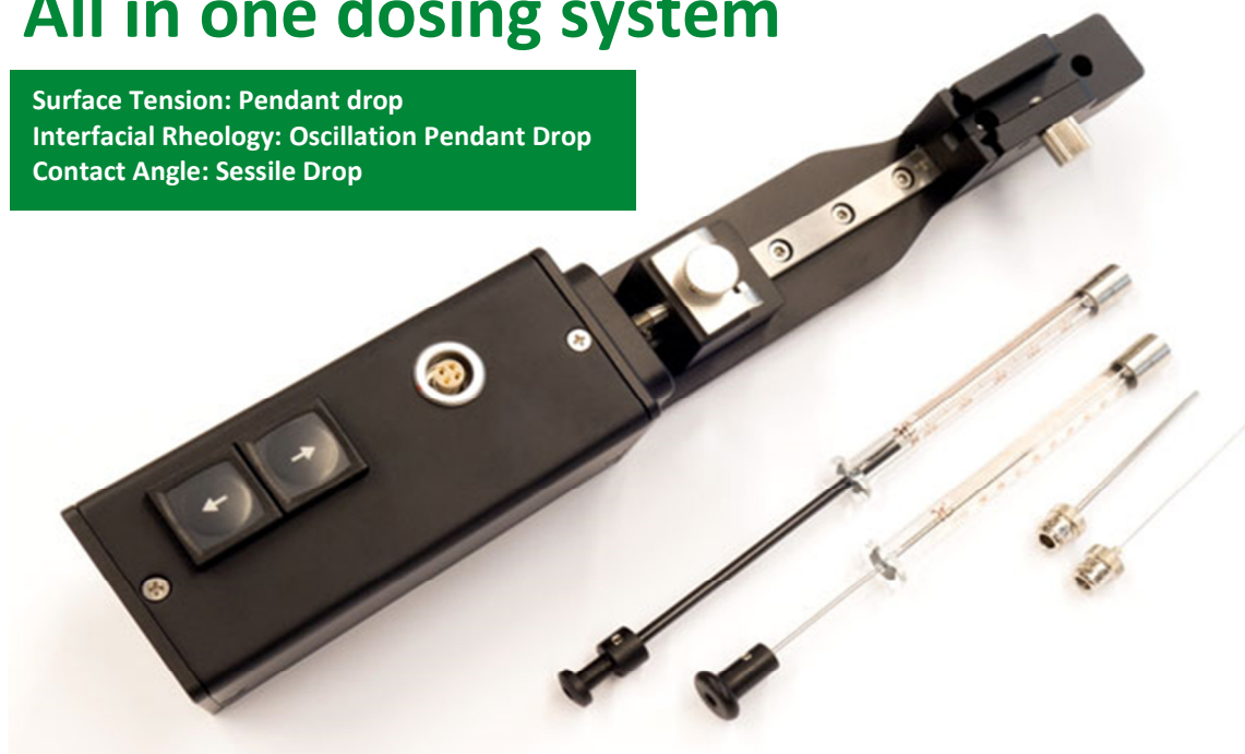
Figure 1: ESr-O a versatile syringe module with precisely controllable back and forth piston speed for oscillation and dosing.
